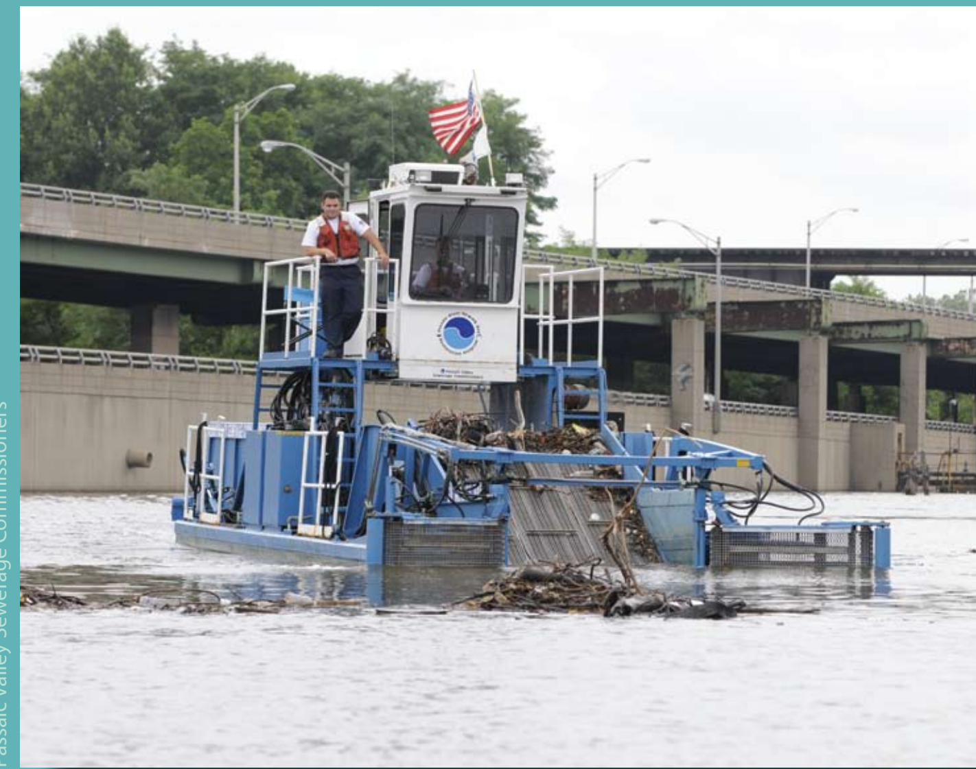
A skimmer boat removes floating trash and debris from the water.
