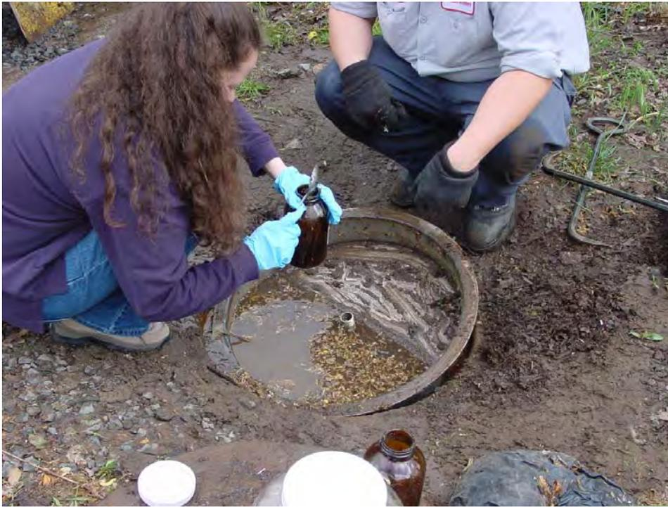
**Figure ES-16. Collection of Storm Water Runoff in the Manhole RLD Insert**
