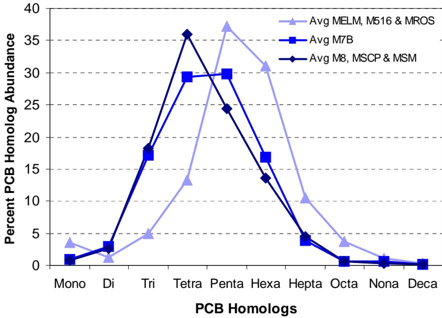
**Figure ES-10. Average PCB Homolog Distributions for Whole Water Samples Collected in Two Rounds From Upstream (Manholes ELM, 516 and ROS), Midstream (Manhole 7B) and Downstream Locations (Manholes SM, SCP and 8) in the Western Sewershed**
