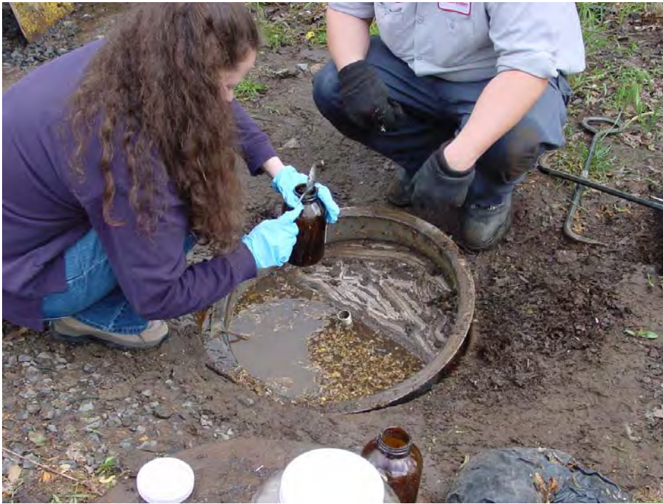
Figure ES-16. Collection of Storm Water Runoff in the Manhole RLD Insert
