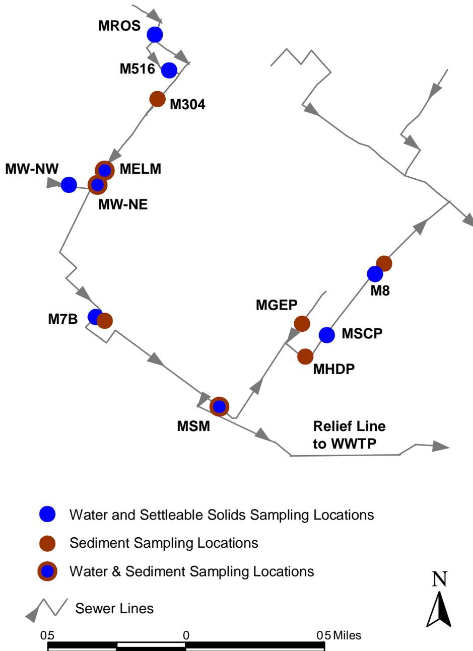
Figure ES-5. LRSA's Western Sewer System and Sampling Locations for Phase IV, Tier 2
